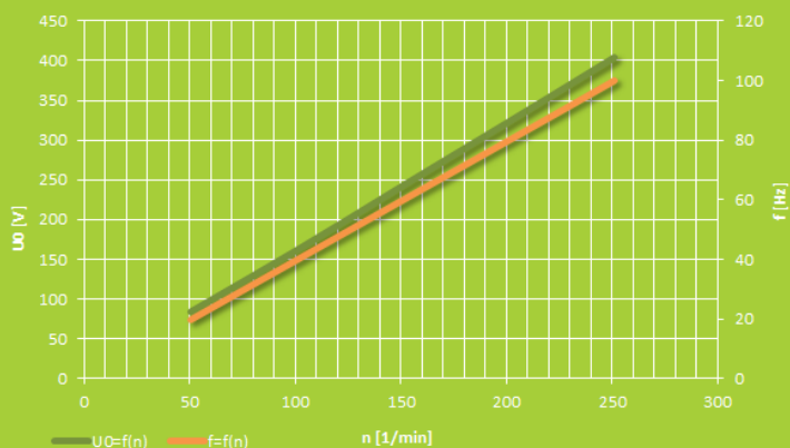
Voltage and frequency dependence on speed for connection with five parallel branches
